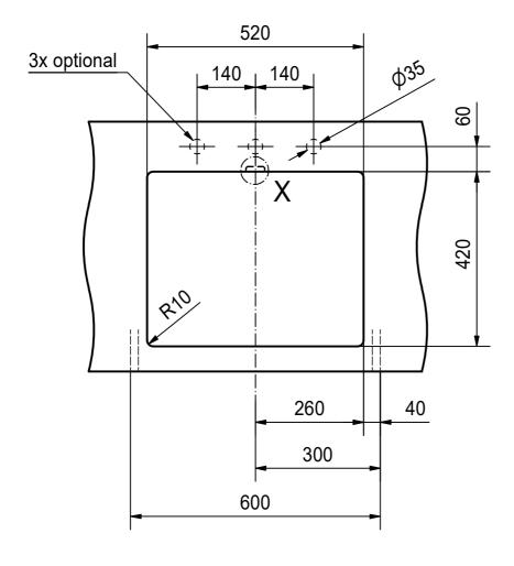
For Inset installation, a recess on the bottom side of the worktop is necessary for the overflow.
