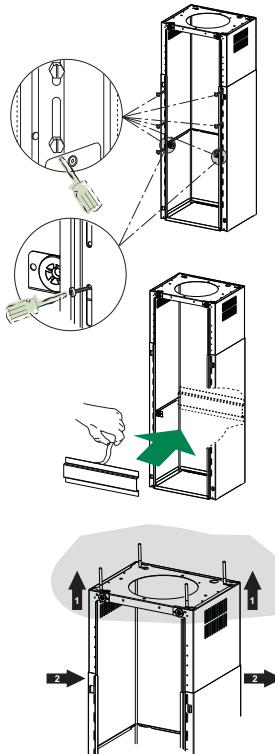
Before final locking of the screws it is possible to make small adjustments to the frame, making sure that the screws do not come out of the adjustment slot.
