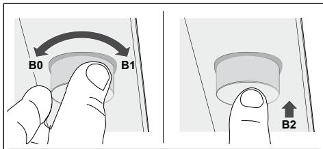
When the dial is turned clockwise the speed increases, passing from:
